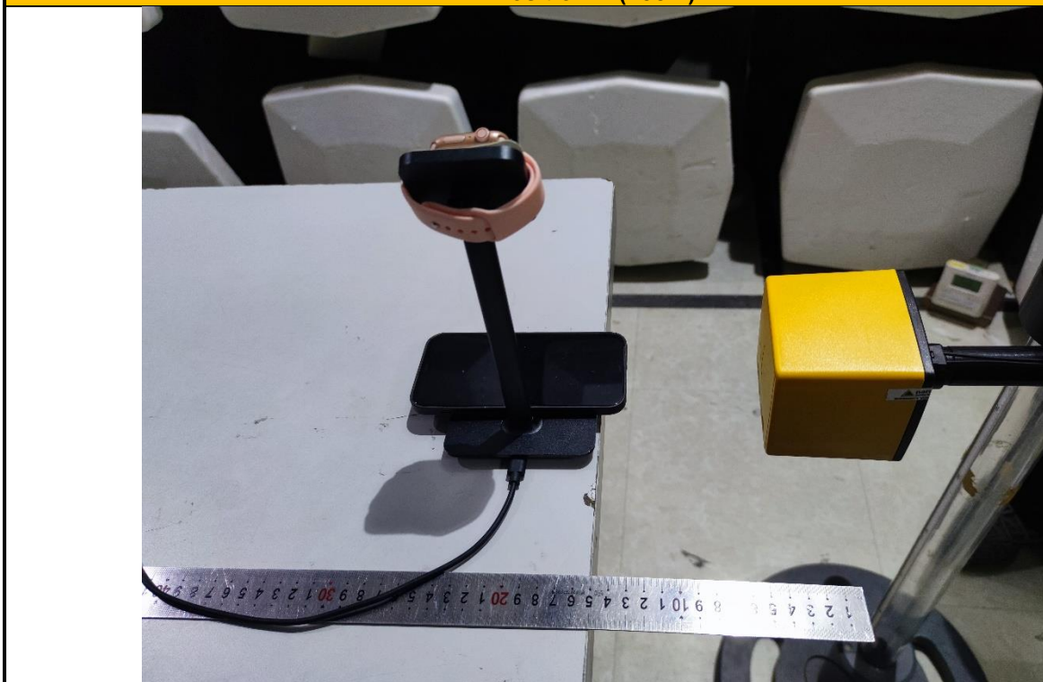
E-Field Strength and H-Field Strength Position B (15cm)
