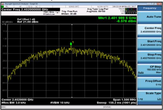
**Power Spectral Density Test Plot (CH-Mid)**
