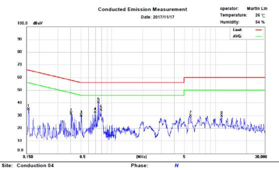
Limit:CISPR22 Class B Conduction(QP)
