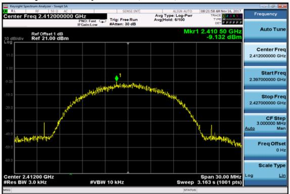
**Power Spectral Density Test Plot (CH-Mid)**
