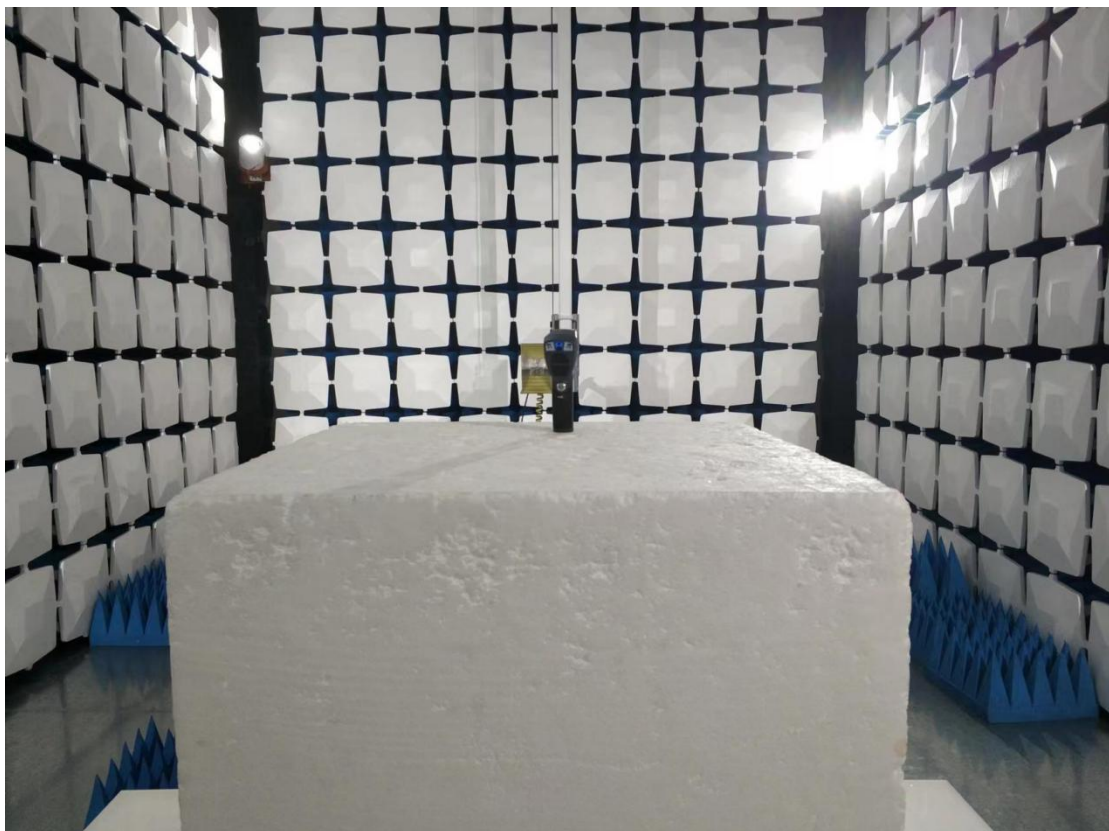
Above 1GHz for radiated emission test setup
