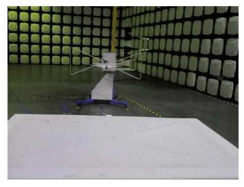
1.1 Field Strength of the Fundamental Signal (15.249(a)) Test Setup
