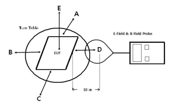
Note: Measurements should be made from all sides and the top of the primary/client pair, with the 10cm measured from the center of the probe(s) to the edge of the device.
