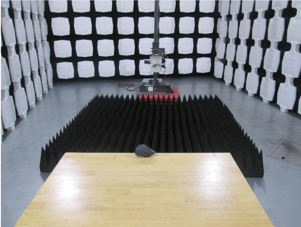
Figure 4 Radiated emission above 1GHz test setup (Motor running and receiving mode)
