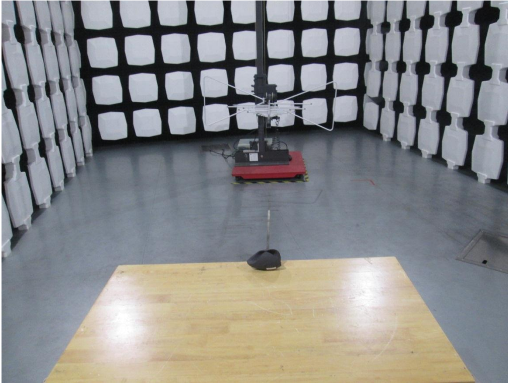
Figure 3 Radiated emission below 1GHz test setup (Motor running and receiving mode)
