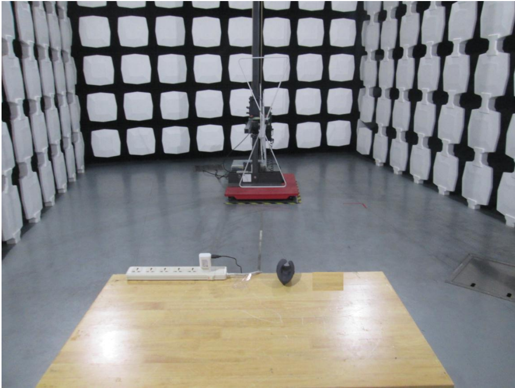
Figure 2 Radiated emission below 1GHz test setup (Charging mode)
