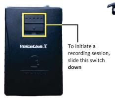
To *start* a recording, slide the VLX switch *down*. The unit will vibrate *once*, indicating that you have successfully initiated a recording. To *stop* a VLX initiated recording, press from the Flashback monitor or DVR. The unit will vibrate *twice*, indicating that you have successfully ended the recording.
