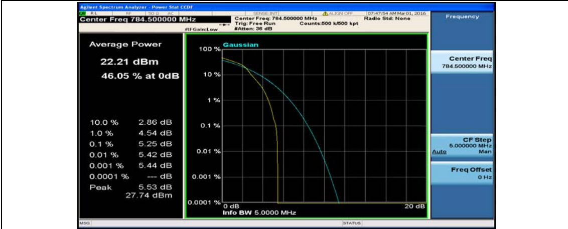
(Channel Bandwidth: 5 MHz)_HCH_16QAM_1RB#24
