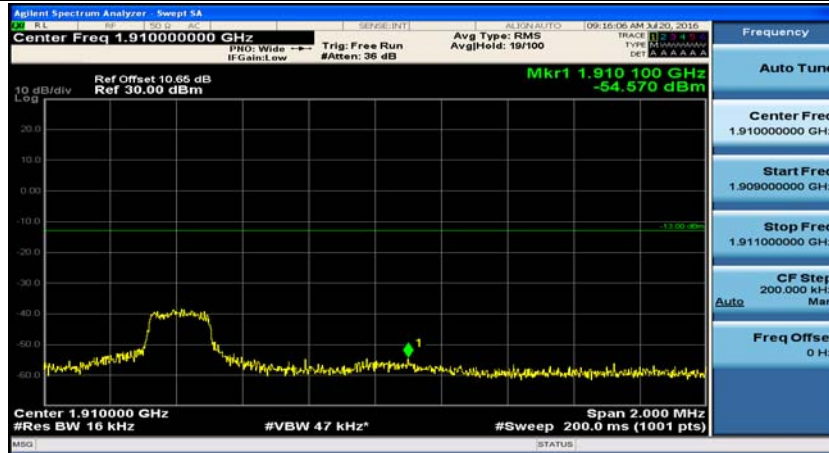
Channel Bandwidth: 10 MHz_HCH_16QAM_1RB#24
