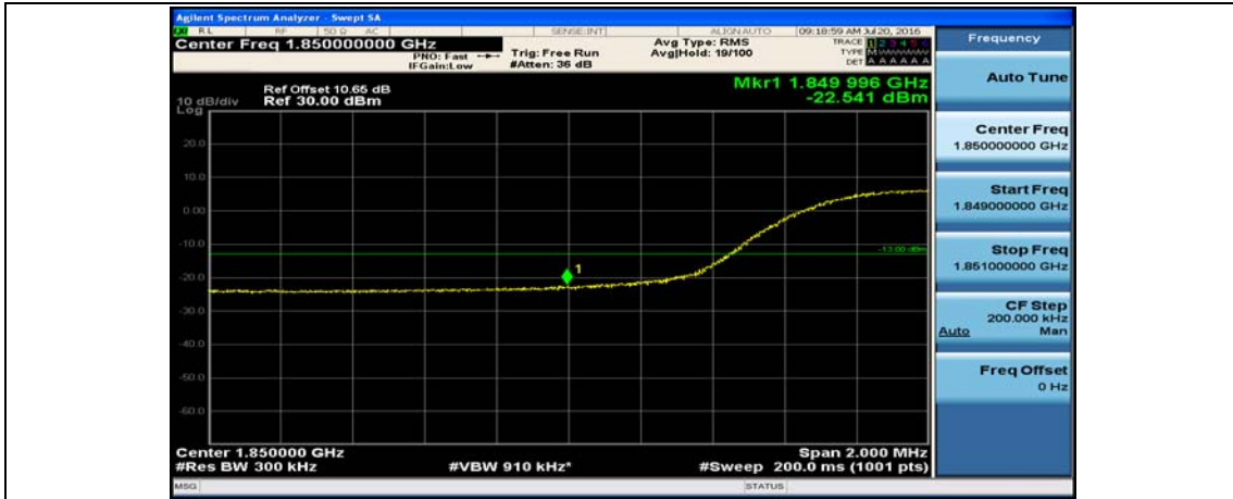
(Channel Bandwidth:15 MHz)_HCH_16QAM_1RB#0
