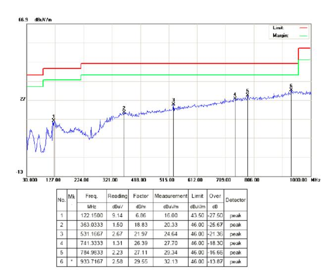
Note: 1. level= Reading level+ Factor, Margin=Measurement-Limit
