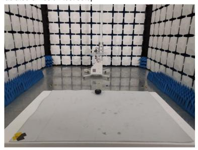
Above 1GHz for radiated emission test setup
