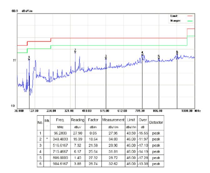
Note: 1. level= Reading level+ Factor, Margin=Measurement-Limit
