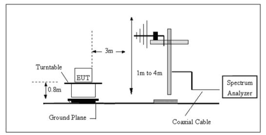
(C) Radiated Emission Test-Up Frequency Above 1GHz
