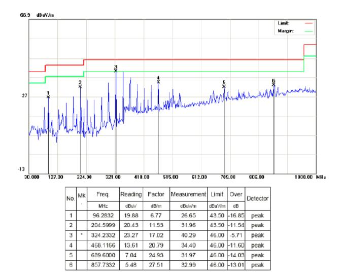
Note: 1. level= Reading level+ Factor, Margin=Measurement-Limit
