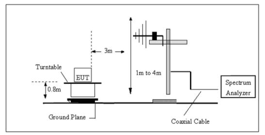
(C) Radiated Emission Test-Up Frequency Above 1GHz
