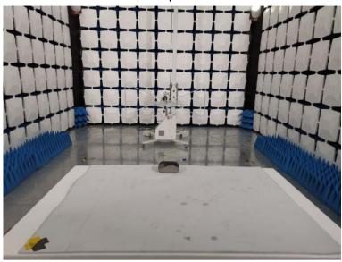
Above 1GHz for radiated emission test setup
