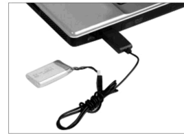
6. Insert the USB charging port into the computer for charging. (The light is off when charging. After charge full, the light is on)
