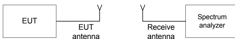
Figure 7.2.1 Occupied bandwidth test setup
