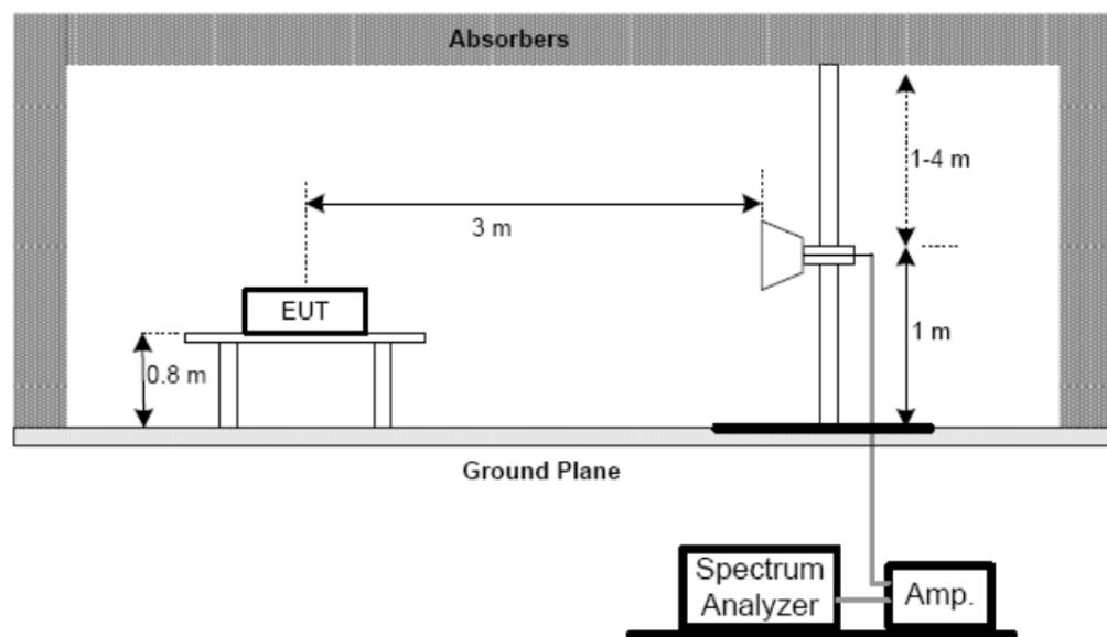
(C) For radiated emissions below 30MHz
