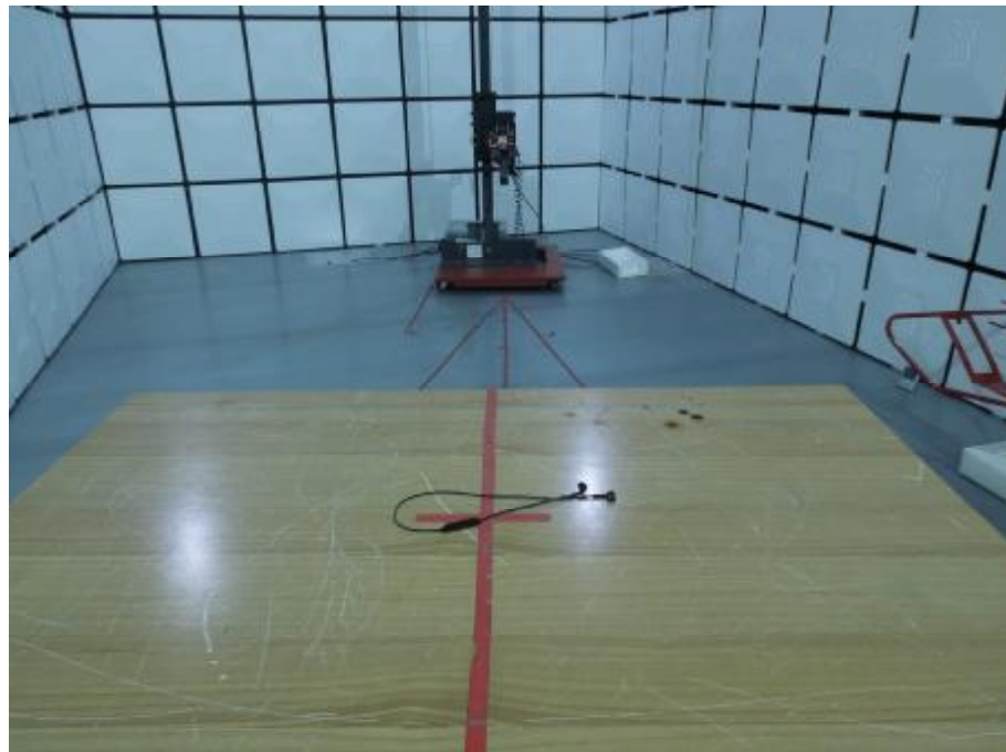
Radiation Test Setup (Above 1 GHz)
