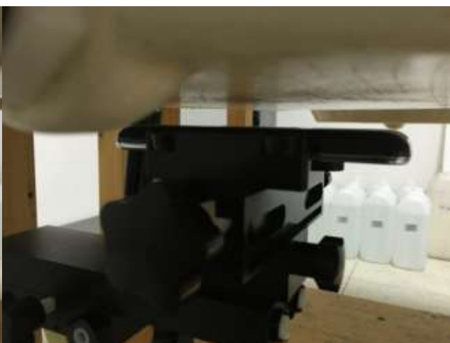
Back of the EUT with 1.5 cm Gap
