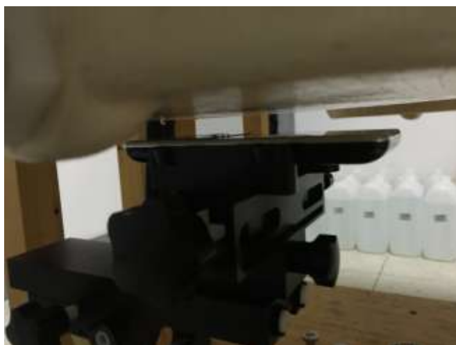
Front of the EUT with 1.5 cm Gap
