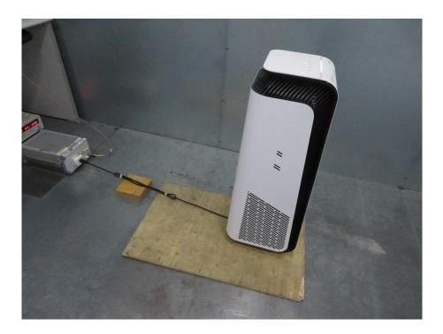
Radiated Emission (9kHz-30MHz)
