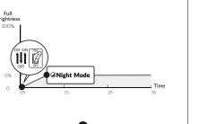
Option 2: Entering into Night Mode when the bulb is ON. While the bulb is ON, quickly flick the switch OFF/ON to start dimming the light bulb. The brightness will automatically stop at the 5% brightness level, Night Mode.
