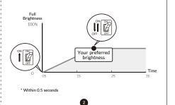
Scenario 2: Adjusting the brightness when the bulb is already ON. Quickly\* flick the switch OFF/ON to initiate dimming of the bulb while it is ON. Then, quickly flick the switch OFF/ON
