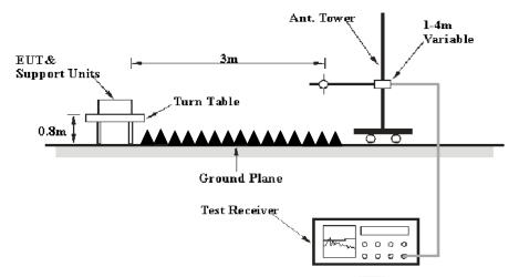
The radiated emission tests were performed in the 3 meters chamber test site, using the setup accordance with the ANSI C63.4-2009. The specification used was the FCC 15.209, and FCC 15.247 limits. The external I/O cables were draped along the test table and formed a bundle 30 to 40 cm long in the middle.
