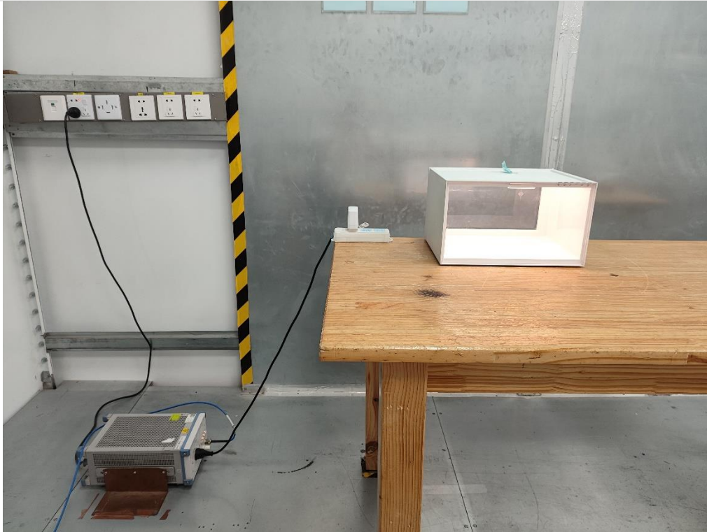
AC Power Line Conducted Emission
