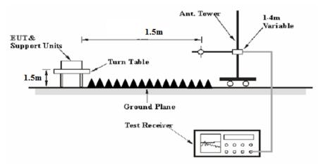
The radiated emission tests were performed in the10 meters chamber for the range 30MHz to 1GHz and the 3 meters chamber B test site for above 1GHz, using the setup accordance with the ANSI C63.10-2013. The specification used was the FCC 15.209, FCC 15.249 and RSS-210, RSS-Gen limits.
