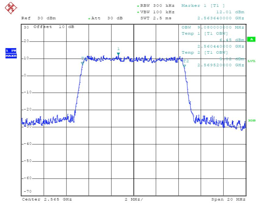
**QPSK (15.0 MHz) - 99% Occupied Bandwidth, Low channel**
