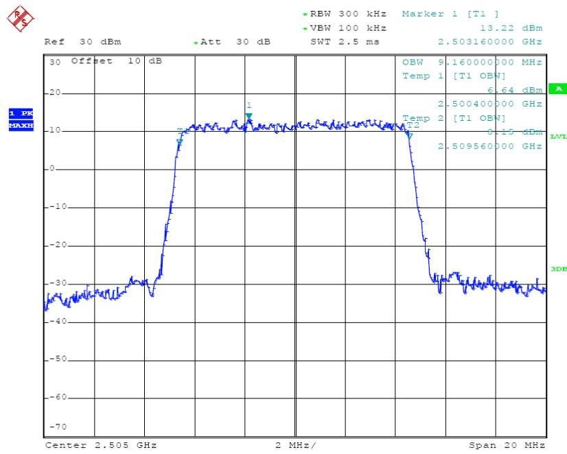
**QPSK (10.0 MHz) - 99% Occupied Bandwidth, Middle channel**
