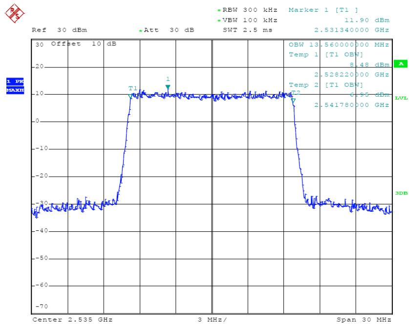
**QPSK (15.0 MHz) - 99% Occupied Bandwidth, High channel**
