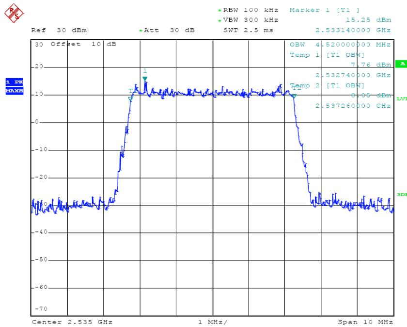
**QPSK (5.0 MHz) - 99% Occupied Bandwidth, High channel**
