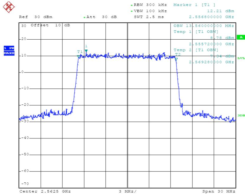
**16-QAM (15.0 MHz) - 99% Occupied Bandwidth, Low channel**
