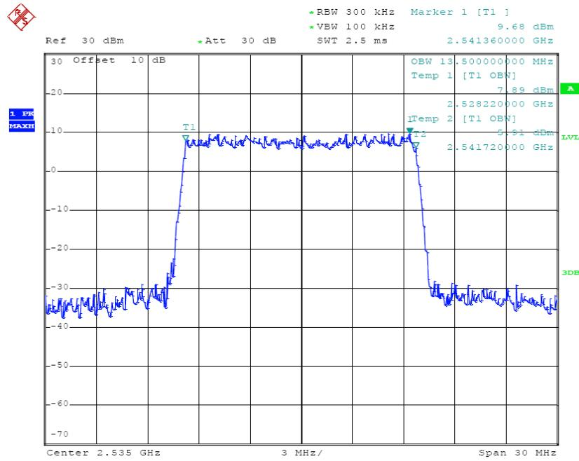
**16-QAM (15.0 MHz) - 99% Occupied Bandwidth, High channel**
