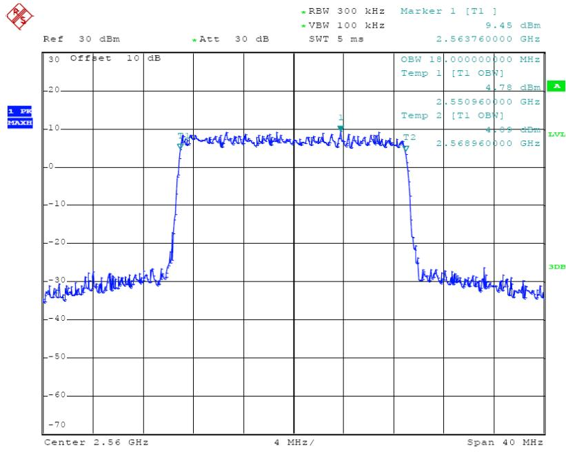
**QPSK (5.0 MHz) - 26 dB Bandwidth, Low channel**
