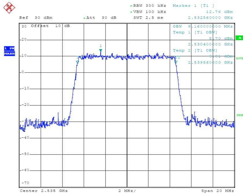
**16-QAM (10.0 MHz) - 99% Occupied Bandwidth, High channel**
