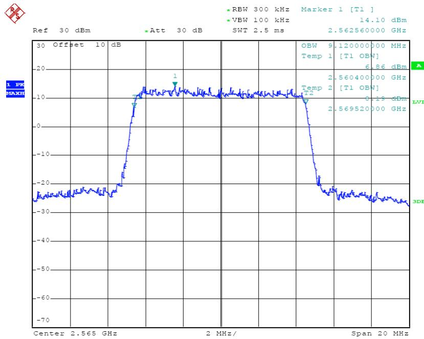
**16-QAM (10.0 MHz) - 99% Occupied Bandwidth, Low channel**
