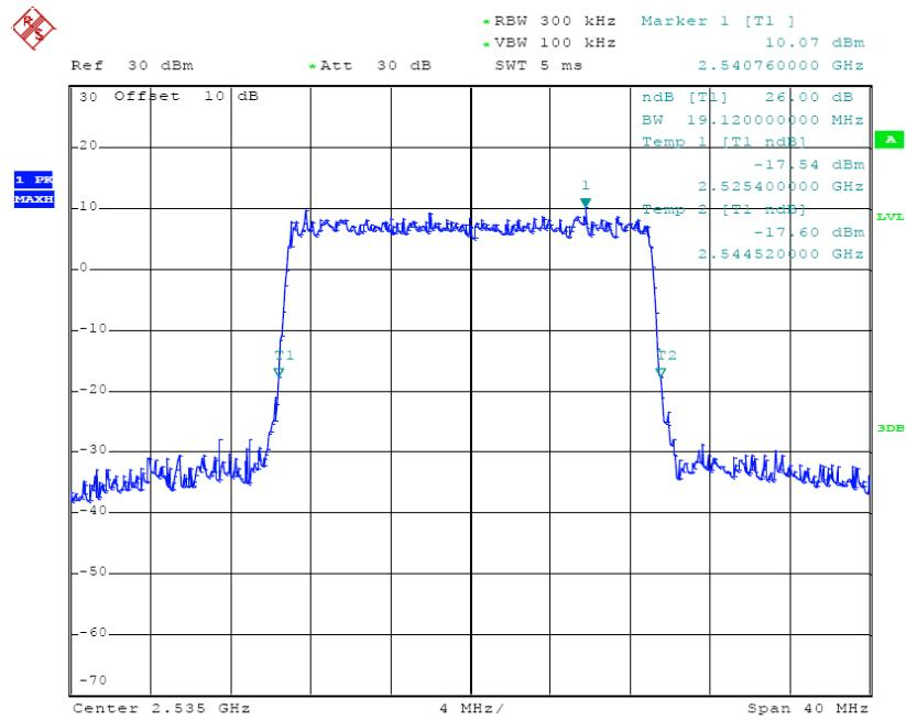
**16-QAM (20.0 MHz) - 26 dB Bandwidth, High channel**
