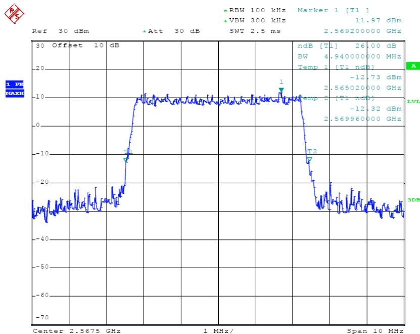
**QPSK (10.0 MHz) - 26 dB Bandwidth, Low channel**
