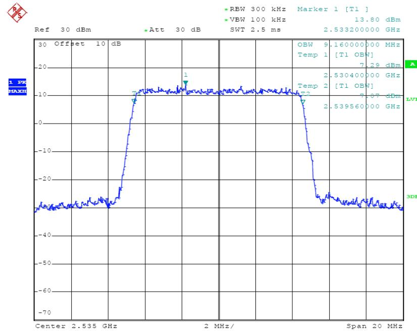
**QPSK (10.0 MHz) - 99% Occupied Bandwidth, High channel**
