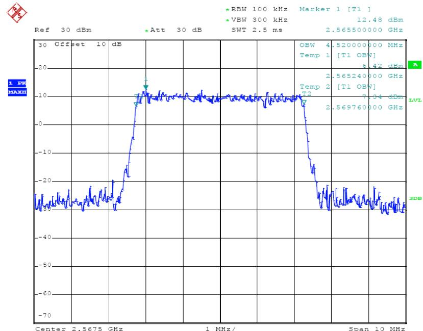
**QPSK (10.0 MHz) - 99% Occupied Bandwidth, Low channel**
