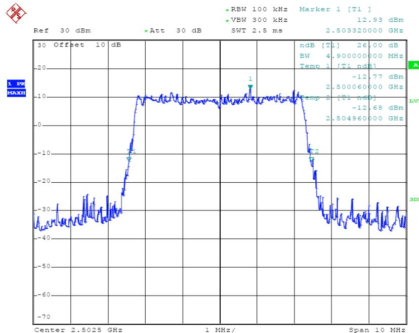
**16-QAM (5.0 MHz) - 26 dB Bandwidth, Middle channel**
