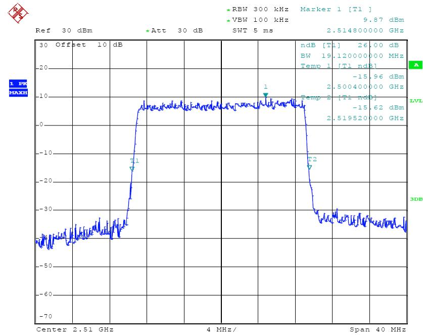
**16-QAM (20.0 MHz) - 26 dB Bandwidth, Middle channel**
