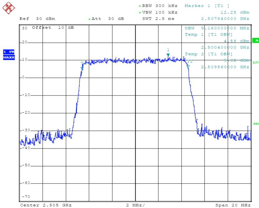
**16-QAM (10.0 MHz) - 99% Occupied Bandwidth, Middle channel**
