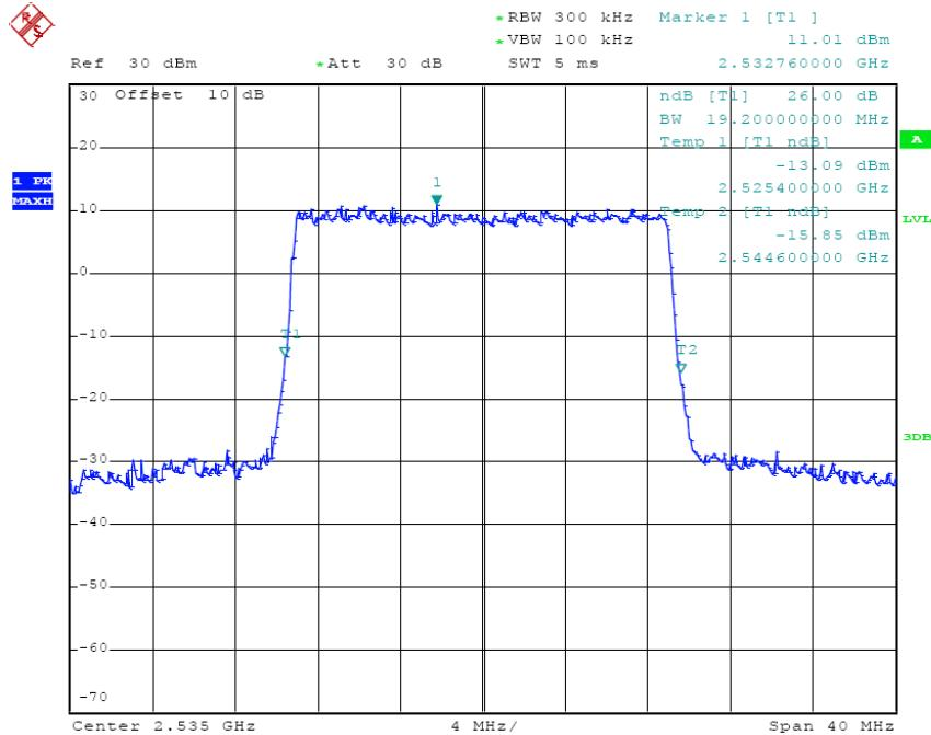
**QPSK (20.0 MHz) - 26 dB Bandwidth, High channel**
