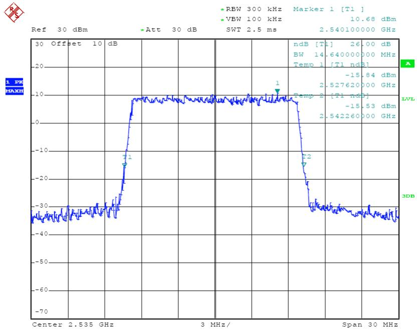
**QPSK (15.0 MHz) - 26 dB Bandwidth, High channel**
