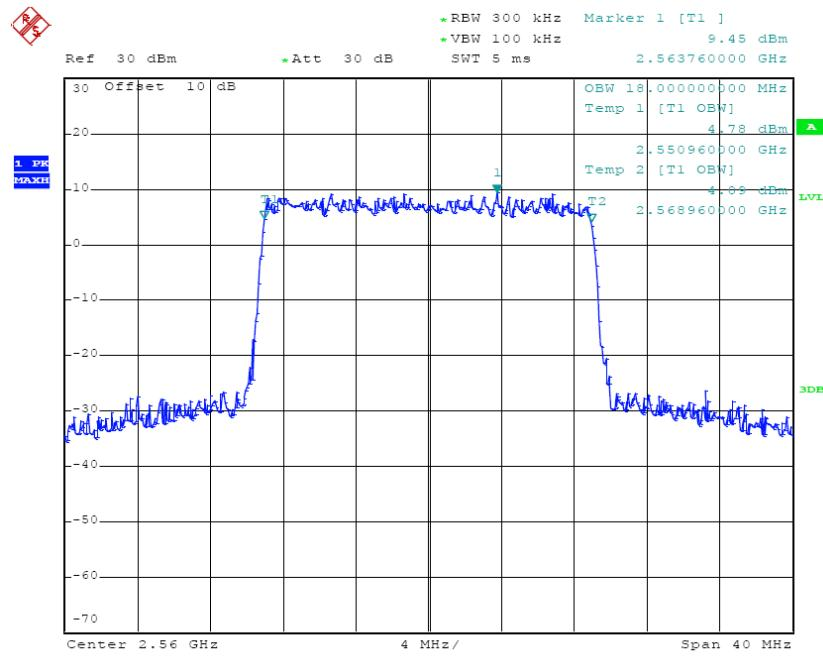
**16-QAM (20.0 MHz) - 99% Occupied Bandwidth, Low channel**
