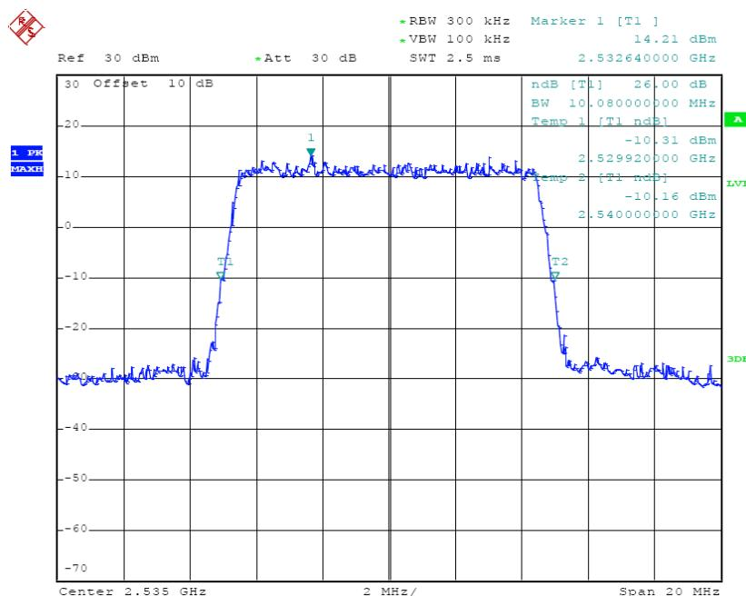
**QPSK (10.0 MHz) - 26 dB Bandwidth, High channel**
