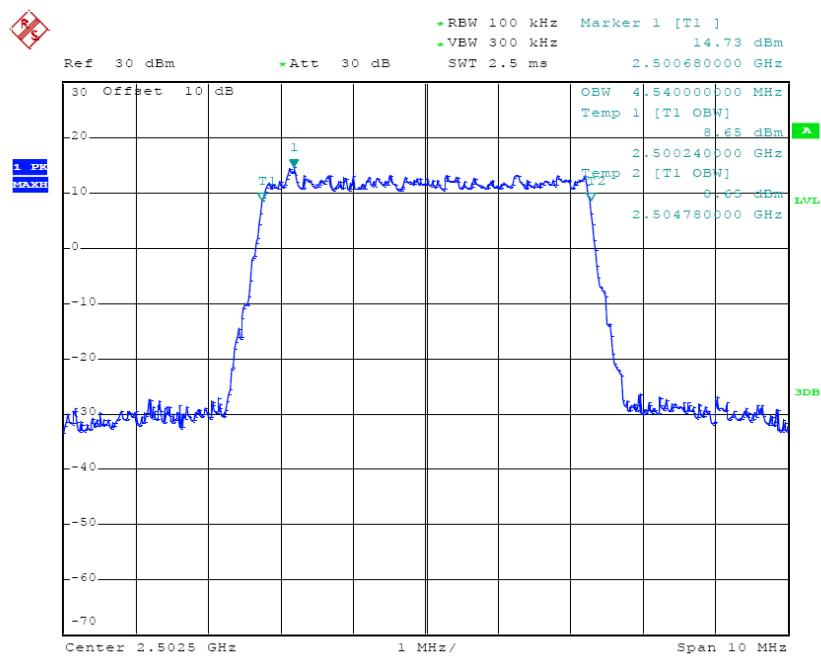
**QPSK (5.0 MHz) - 99% Occupied Bandwidth, Middle channel**
