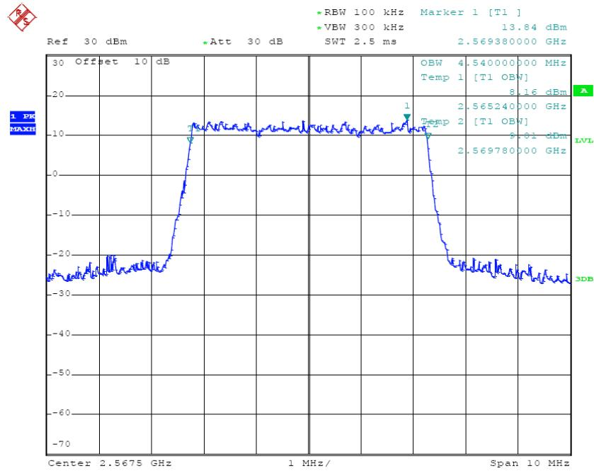
**16-QAM (5.0 MHz) - 99% Occupied Bandwidth, Low channel**
