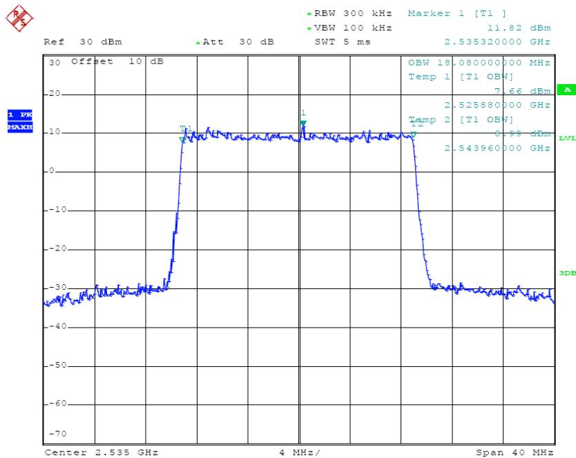
**QPSK (20.0 MHz) - 99% Occupied Bandwidth, High channel**
