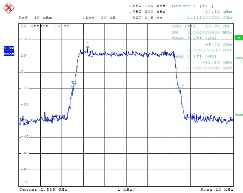
**QPSK (5.0 MHz) - 26 dB Bandwidth, High channel**
