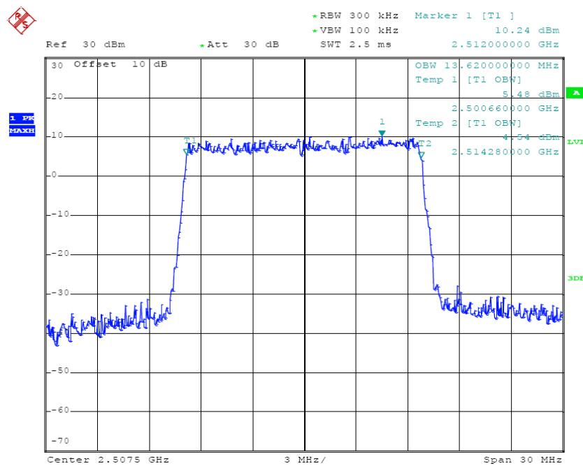
**16-QAM (15.0 MHz) - 99% Occupied Bandwidth, Middle channel**
