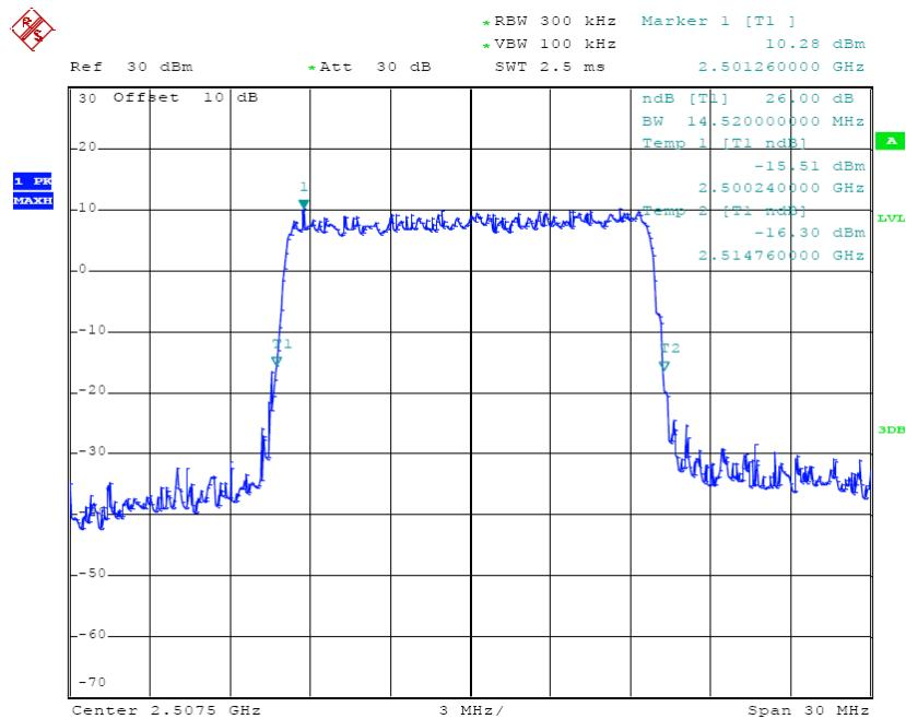
**16-QAM (15.0 MHz) - 26 dB Bandwidth, Middle channel**
