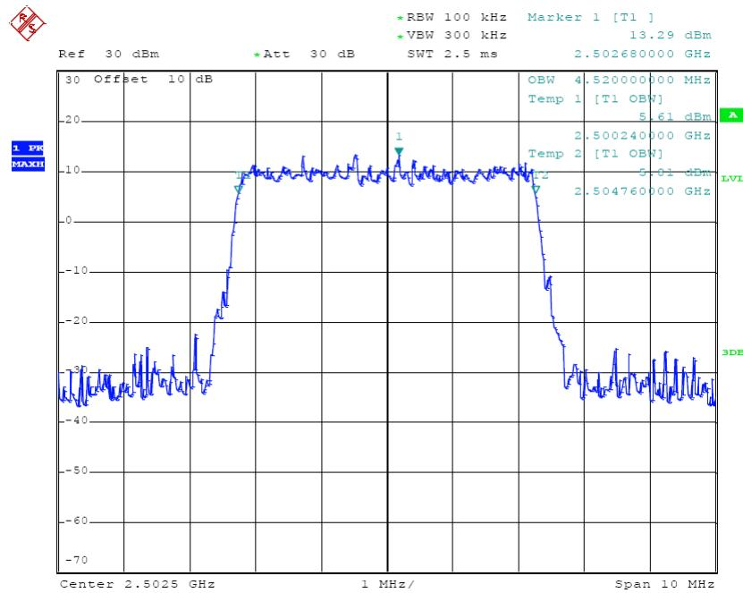
**16-QAM (5.0 MHz) - 99% Occupied Bandwidth, Middle channel**
