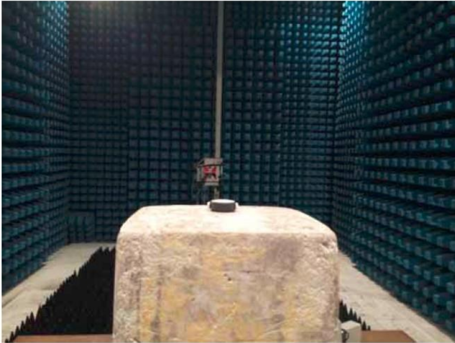
Description: Radiated Emission Test Setup for 1~18GHz
