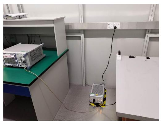
FCC RADIATED EMISSION TEST SETUP
