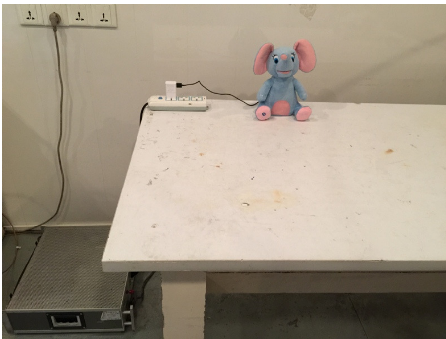
Set-up for Conducted Emission at AC mains power port
