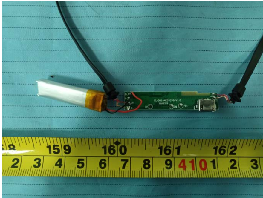
EUT –Main Board & Battery Bottom View
