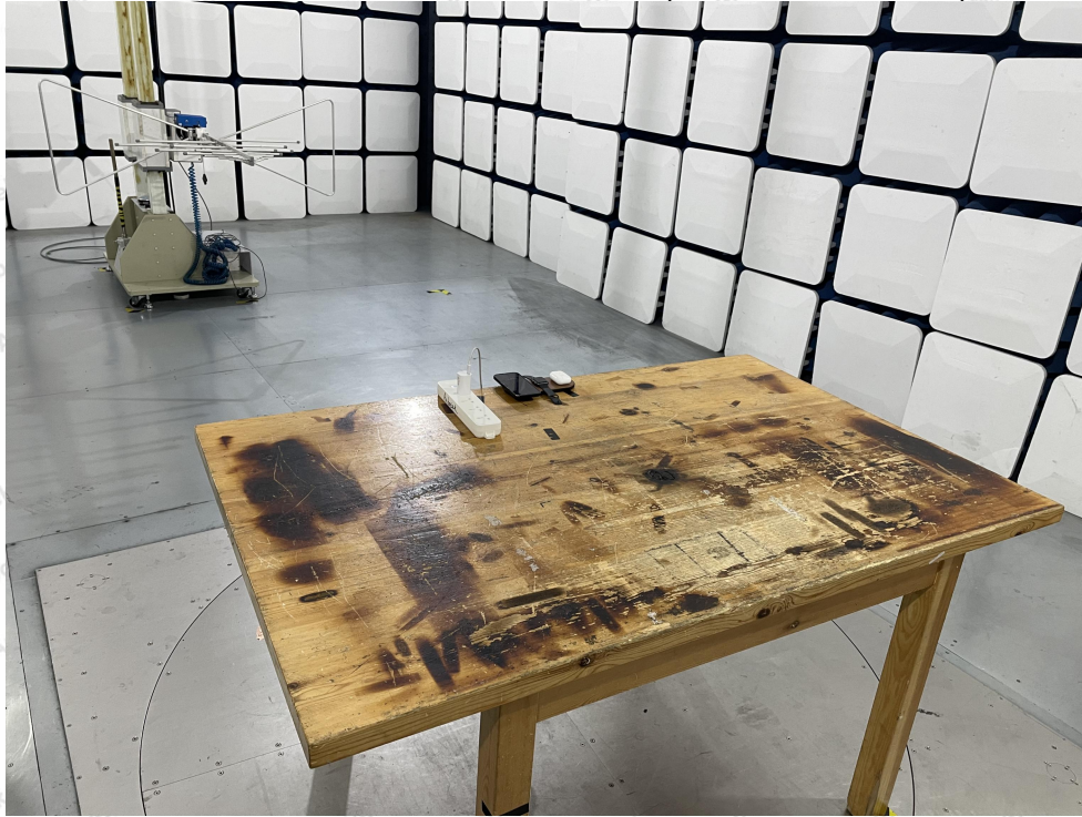
Photo of Radiation Emission Test (30MHz~1000MHz)
