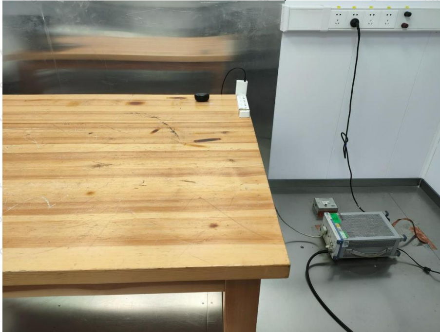
Conducted Emission at AC power line
