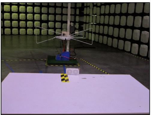
Above 1 GHz: (full anechoic chamber)
