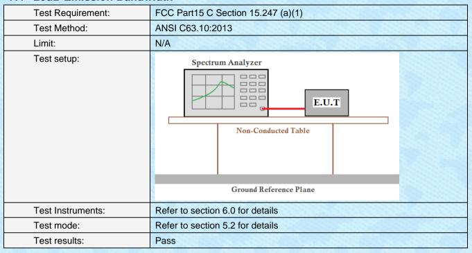
Measurement Data: The detailed test data see Appendix for BT EDR.
