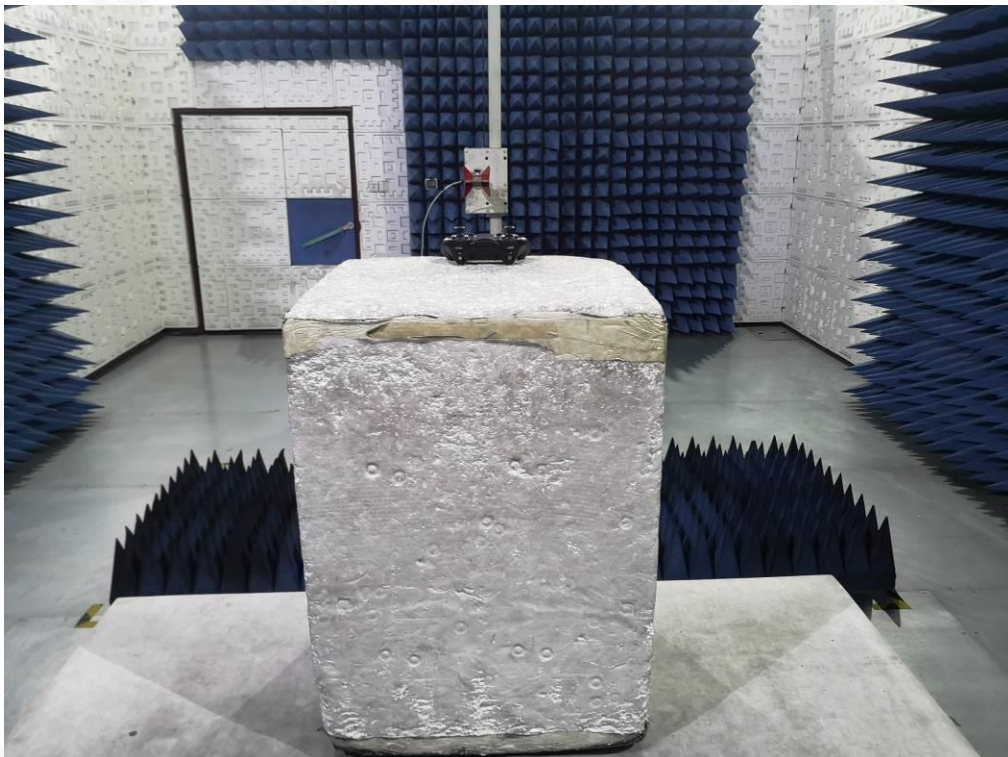
FCC RADIATED EMISSION TEST SETUP ABOVE 1GHZ
