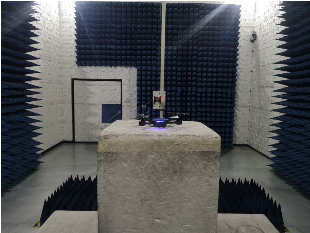
FCC RADIATED EMISSION TEST SETUP ABOVE 1GHZ
