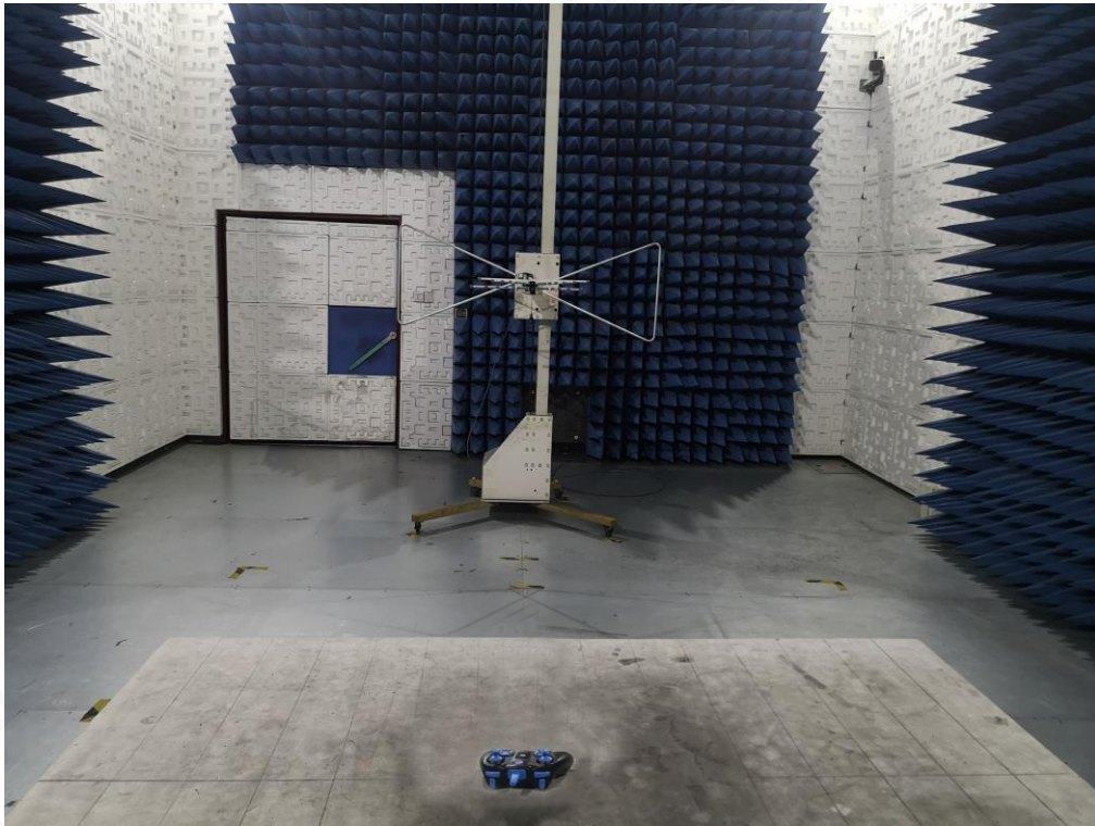
FCC RADIATED EMISSION TEST SETUP ABOVE 1GHZ
