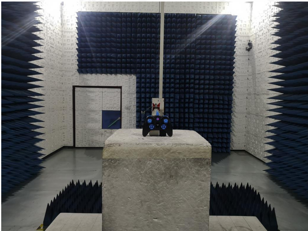
FCC RADIATED EMISSION TEST SETUP ABOVE 1GHZ
