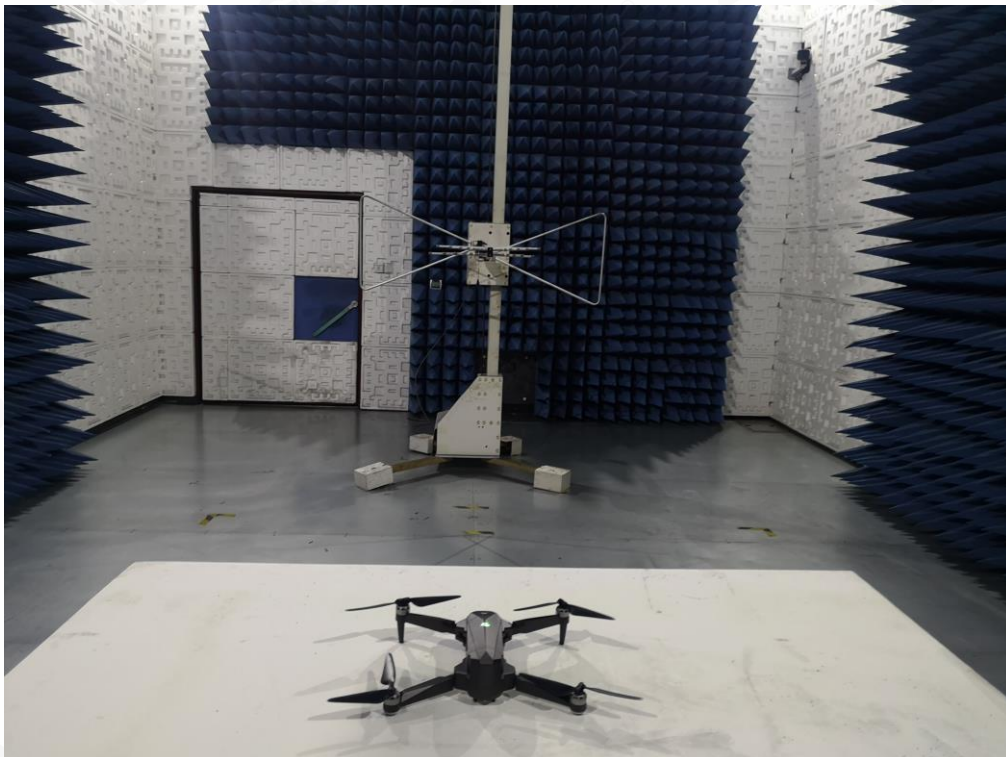
FCC RADIATED EMISSION TEST SETUP BELOW 1GHZ
