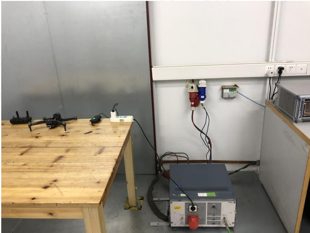
FCC RADIATED EMISSION TEST SETUP BELOW 1GHZ
