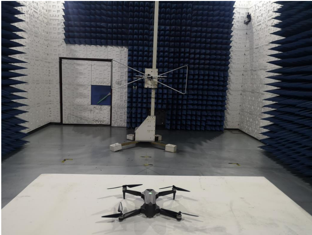
FCC RADIATED EMISSION TEST SETUP BELOW 1GHZ
