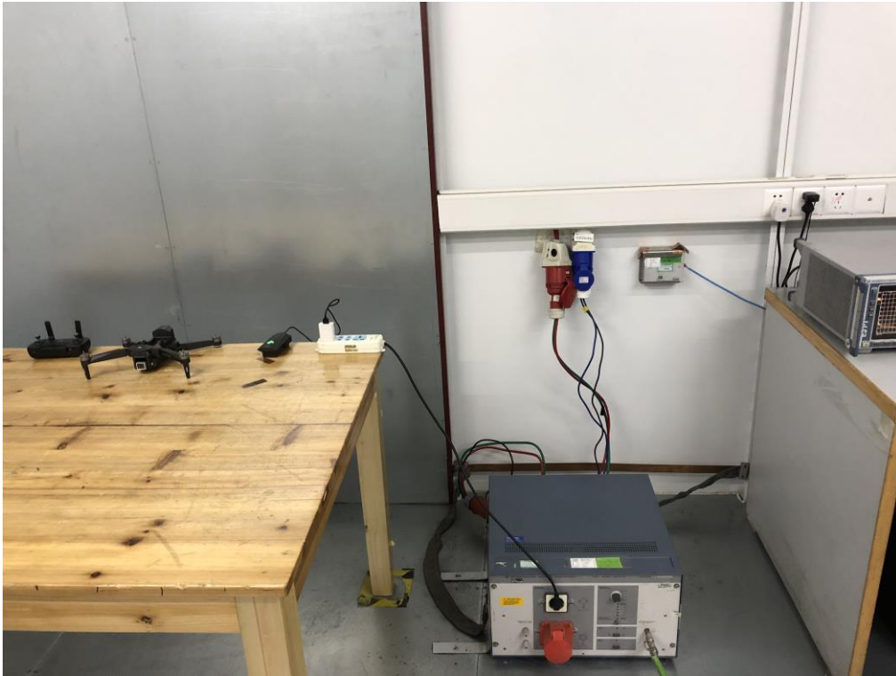
FCC RADIATED EMISSION TEST SETUP BELOW 1GHZ
