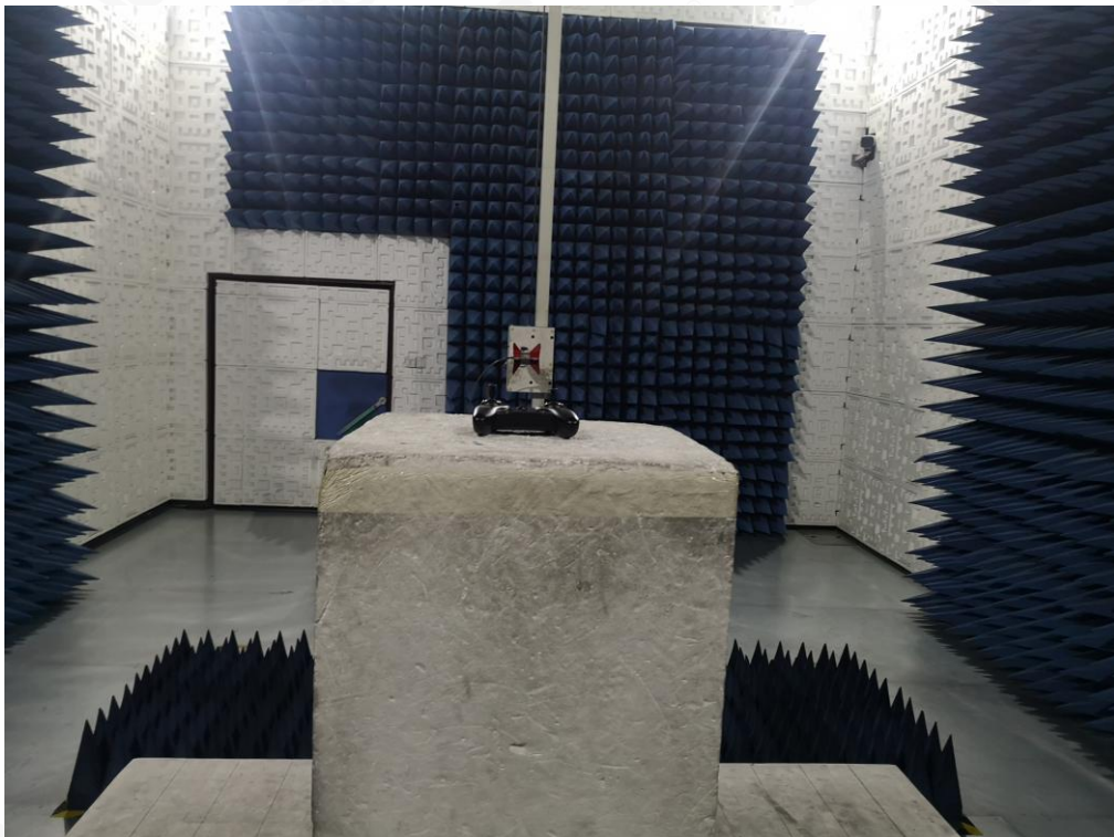
FCC RADIATED EMISSION TEST SETUP ABOVE 1GHZ
