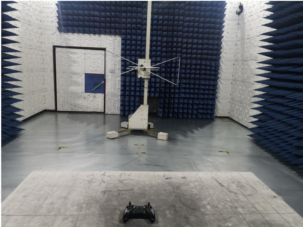
FCC RADIATED EMISSION TEST SETUP ABOVE 1GHZ
