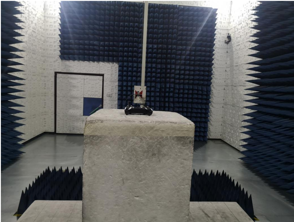
FCC RADIATED EMISSION TEST SETUP ABOVE 1GHZ
