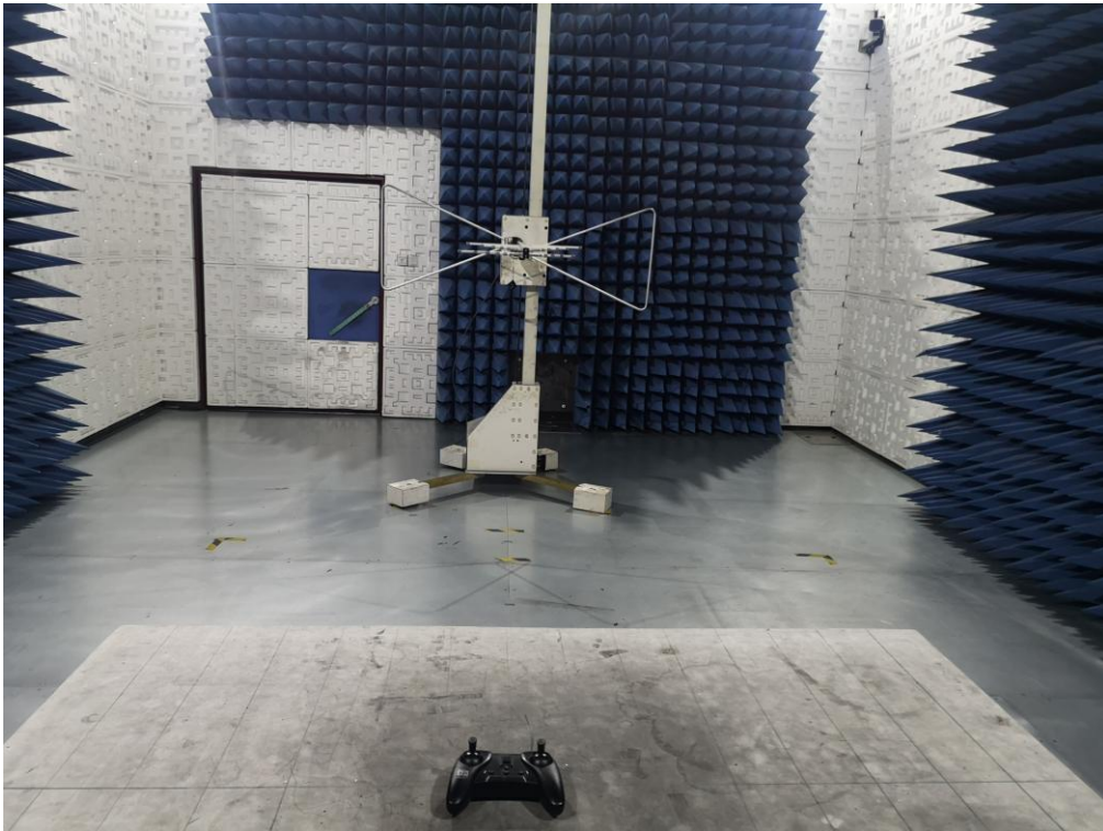
FCC RADIATED EMISSION TEST SETUP ABOVE 1GHZ
