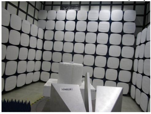
1.2 Radiated Emissions Test Setup
