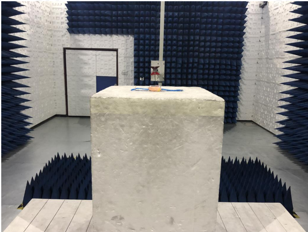
FCC RADIATED EMISSION TEST SETUP ABOVE 1GHZ
