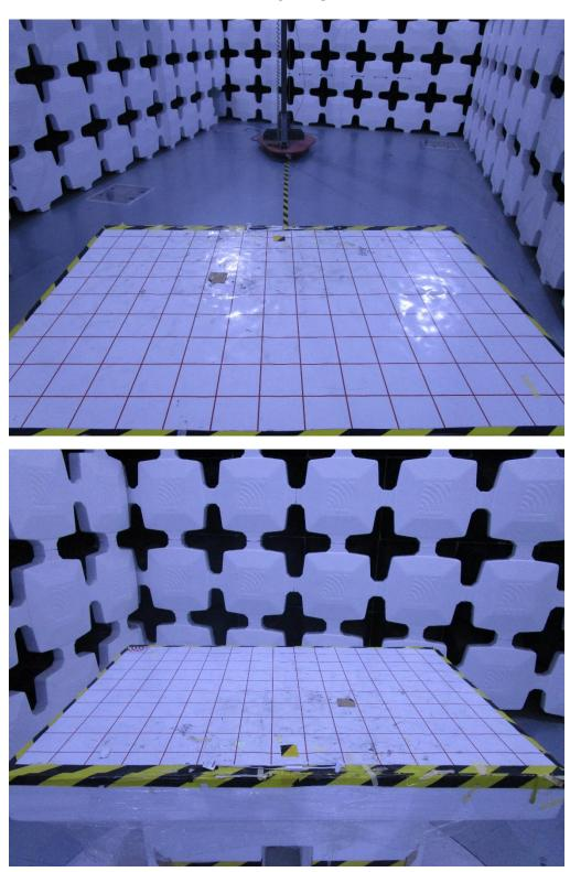
(The EUT is placed at the center of turntable)
