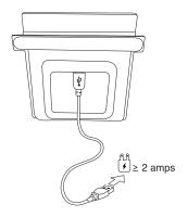
Connect the supplied Micro USB cable to the Wireless Charging Stand's input port and then connect it to a USB-A adapter (2 amps or QC 3.0).
