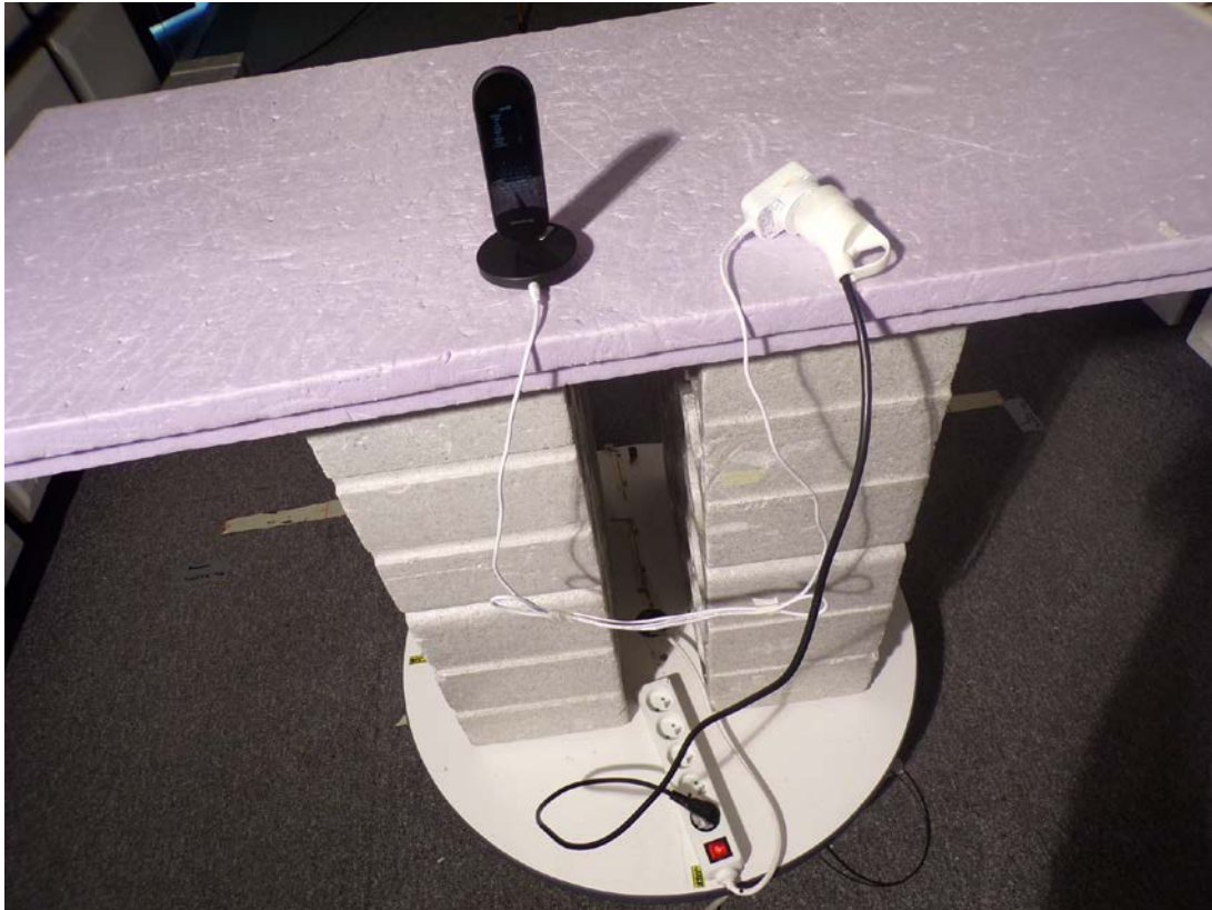
Test setup for radiated emission below 1GHz
