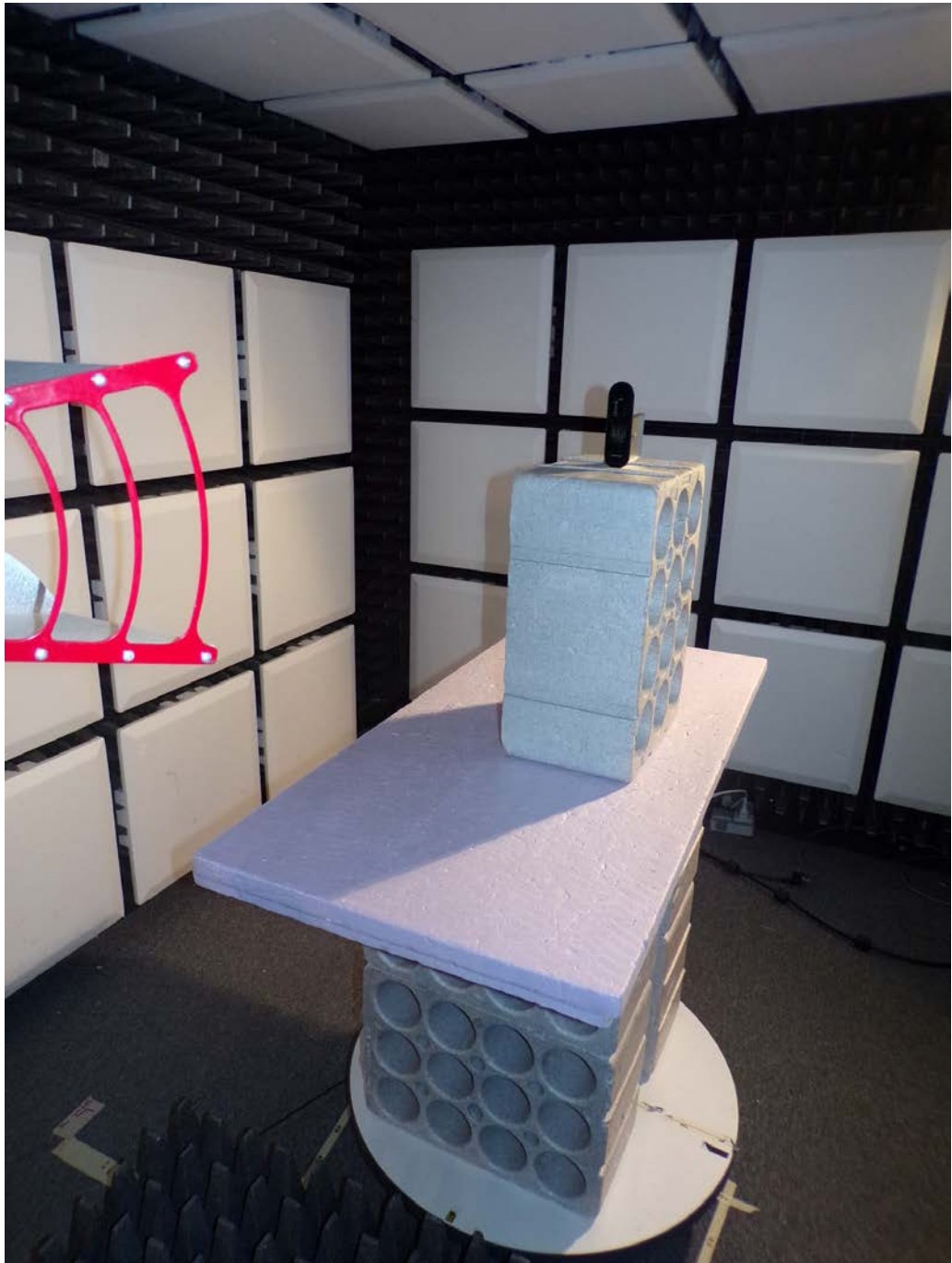
Test setup for radiated emission above 1GHz
