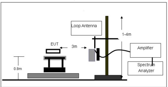
(B) Radiated Emission Test-Up Frequency 30MHz~1GHz
