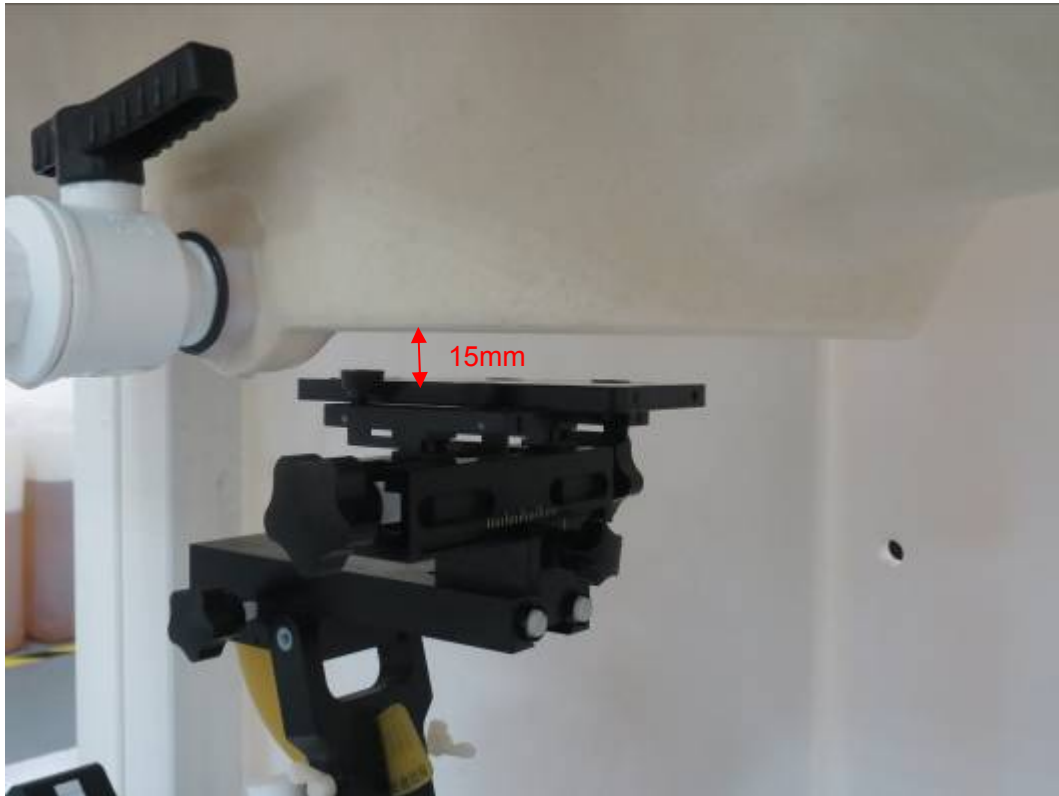
Picture 13: Back Side, the distance from handset to the bottom of the Phantom is 15mm
