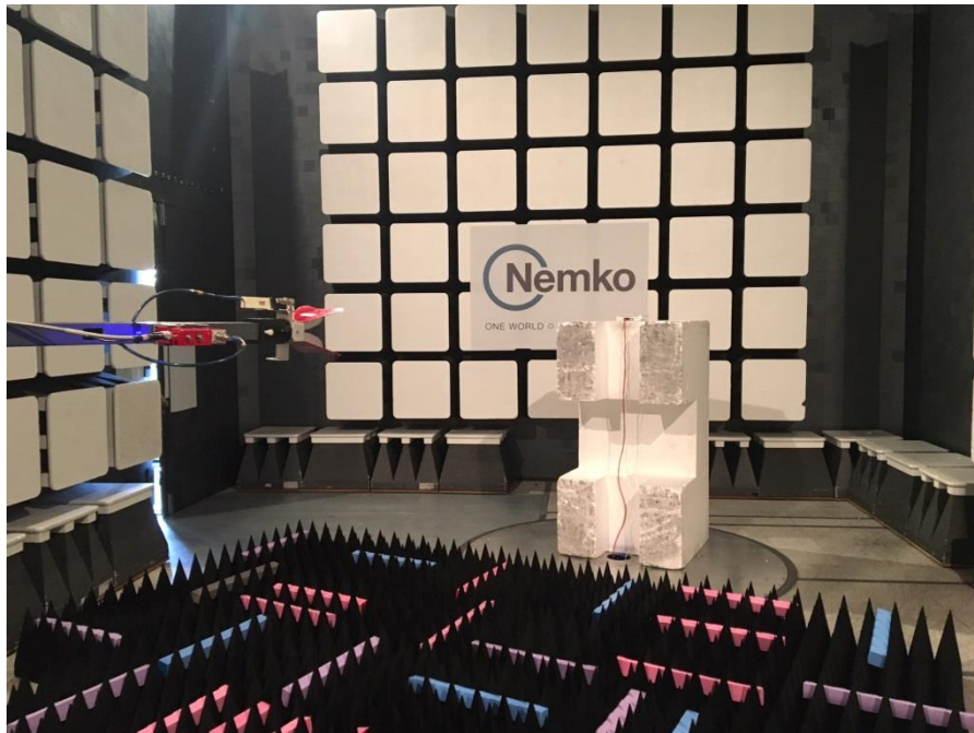
Figure 8.1-19: Radiated – Undesirable (unwanted) emissions setup photo – above 1 GHz
