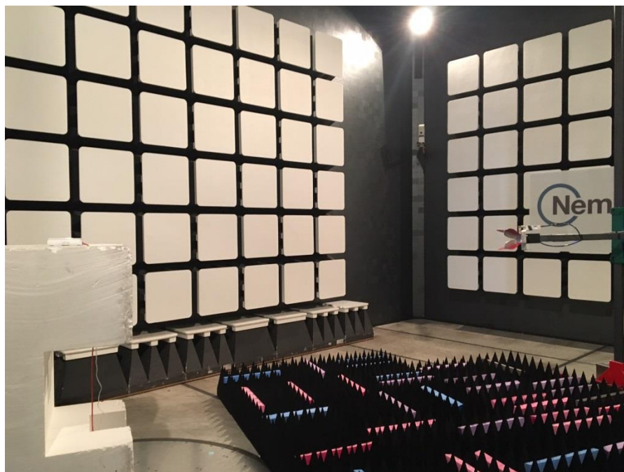
Figure 8.1-18: Radiated – Undesirable (unwanted) emissions setup photo – above 1 GHz
