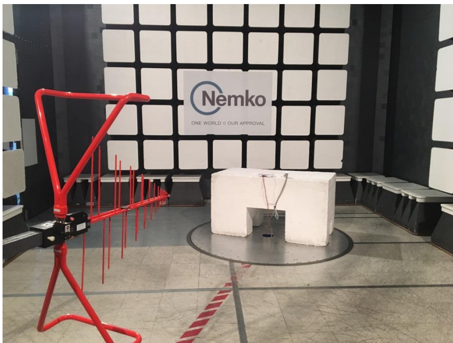
Figure 8.1-16: Radiated – Undesirable (unwanted) emissions setup photo – below 1 GHz
