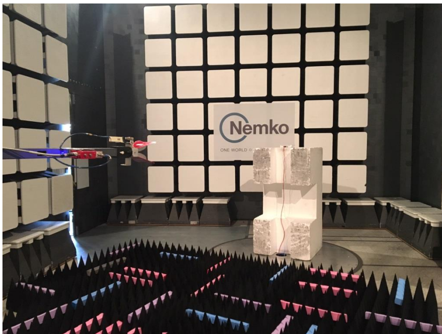
Figure 8.1-30: Radiated – Spurious (out-of-band) unwanted emissions setup photo – above 1 GHz
