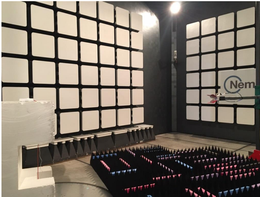
Figure 8.1-29: Radiated – Spurious (out-of-band) unwanted emissions setup photo – above 1 GHz
